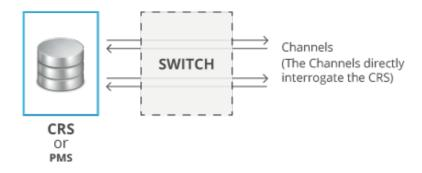
The channels directly interrogate the database of the CRS (or the PMS).
