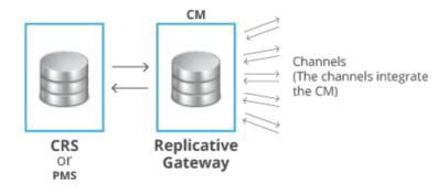
The system replicates the database of the CRS, producing a duplicate designed to absorb the high number of requests per minute of the channels.
